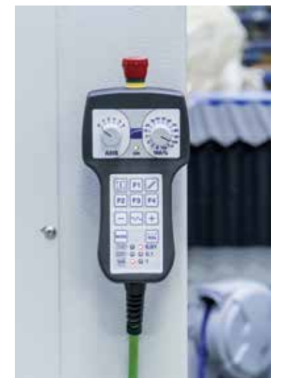
Remote control up to 6 axes that allow you to operate close to the cutting surface and set multi-origins.
