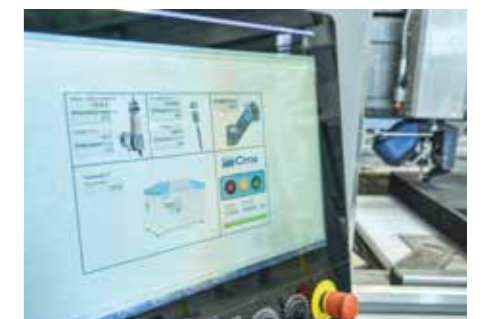
Hardware and Software control of the waterjet cutting system designed to offer the operator a simple and intuitive interface that allows for complete control of all the system functions, including the tapering control (JDC) for 5-axes machines.
