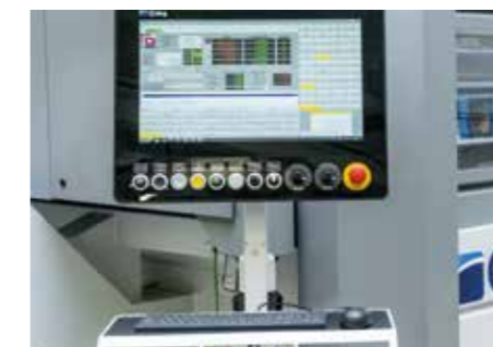
Hardware and Software control of the waterjet cutting system designed to offer the operator a simple and intuitive interface that allows for complete control of all the system functions, including the tapering control (JDC) for 5-axes machines.
