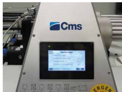
Software-based electronic control of cutting pressure
