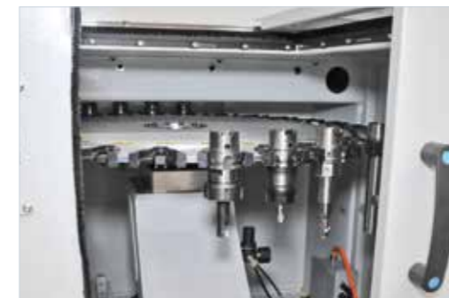
30 stations automatic rotary tool changer
