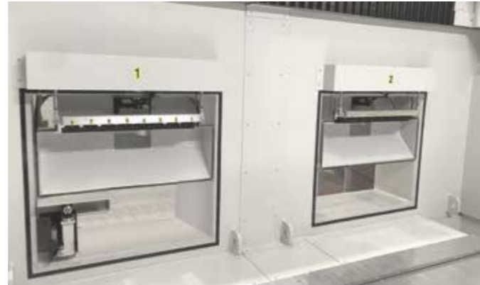
Tool changer magazine; 16 stations
