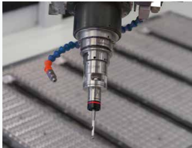
Probe device fitted on the tool holder with transmission via radio signal.
