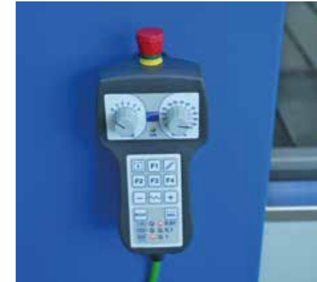
Remote pushbutton pad to control up to 6 axes that allow you to operate close to the cutting surface and set multi-origins.
