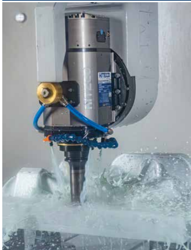
FLOOD COLANT SYSTEM
