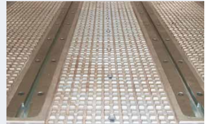
Aluminum vacuum table with T slots
