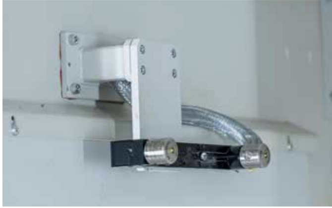
Laser device for measuring tool length and diameter
