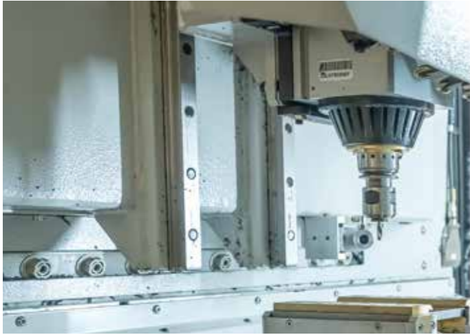
Ionizing bar built into the base and laser to check the tool is present and intact
