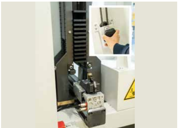
Blank magazine with simplified adjustment
