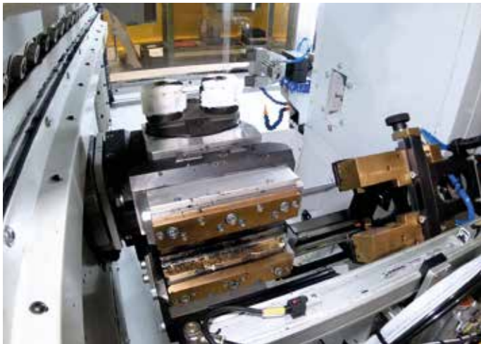
Clamp change device with vertical movement controlled by CN axis and 0-180° rotation
