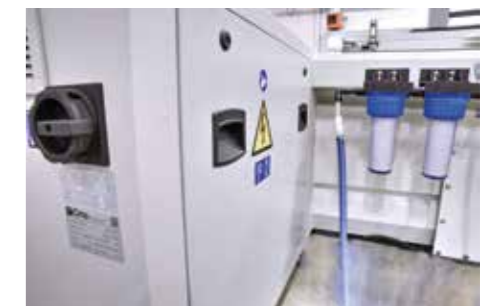
Control panel integrated into the base of the tank to reduce bulk on the ground
