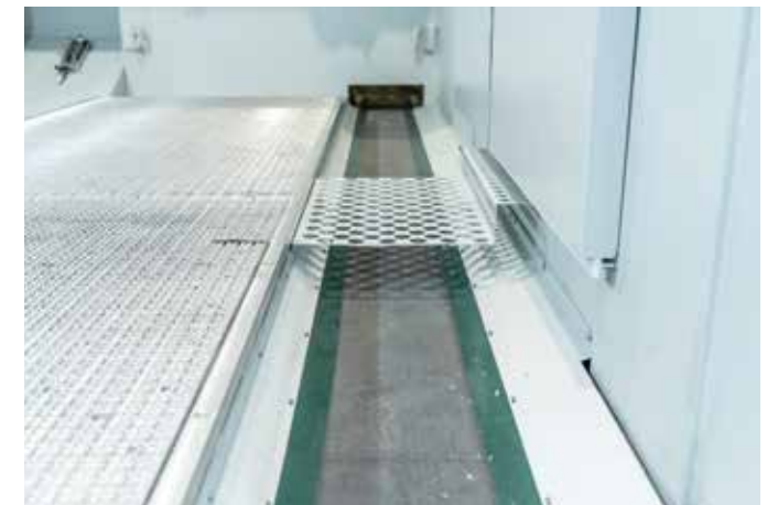
Chips management with integrated conveyor
