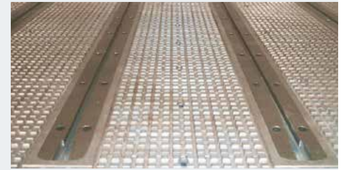
Aluminum vacuum table with T slots
