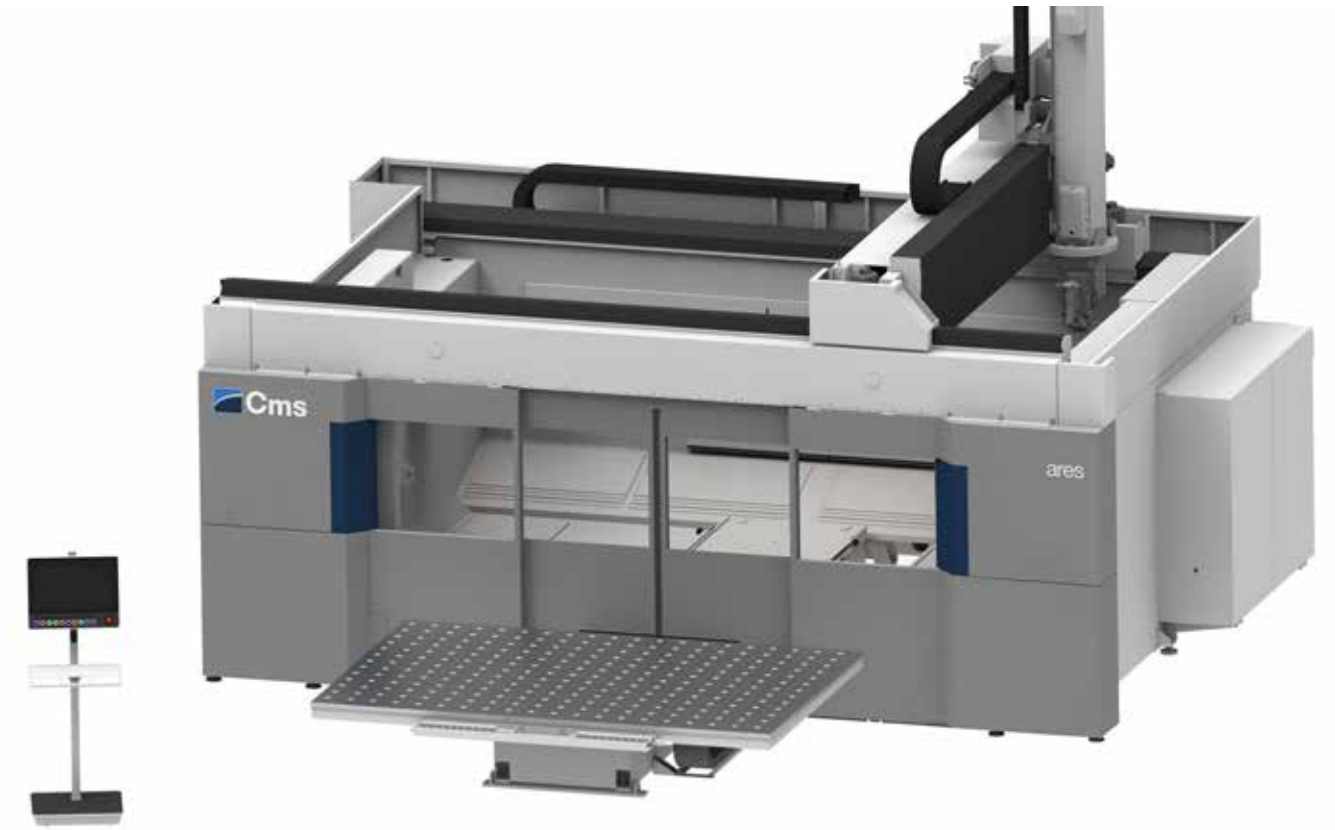
Ares with single extractable working table 1APC (Automatic Pallet Change)
