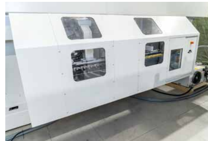
Tool-chain magazine with exchange handgrip
