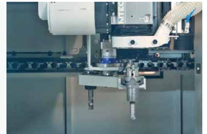
Tool-chain magazine with exchange handgrip
