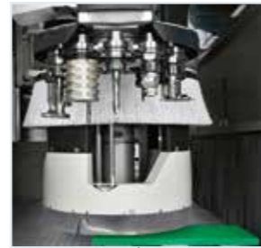
Excellent cleanliness of the machine and its surroundings thanks to the dual coaxial suction hood, which can extract chips and dust under all working conditions.
