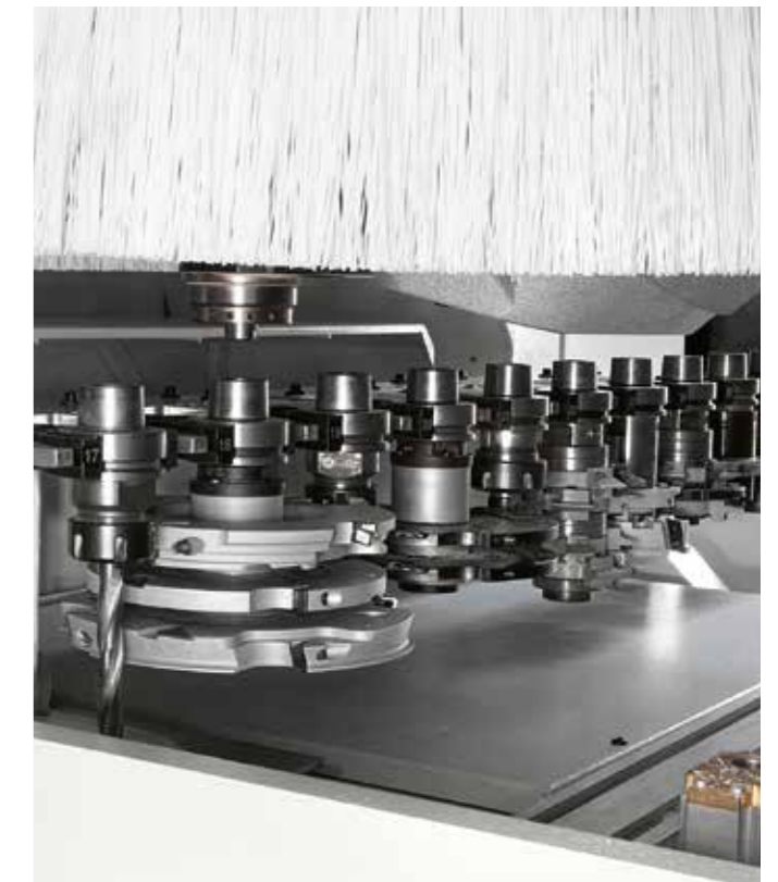
TR 12 12 positions Maximum efficiency with a linear magazine to the right of the worktable.
