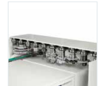
Side magazine with up to 12 positions.
