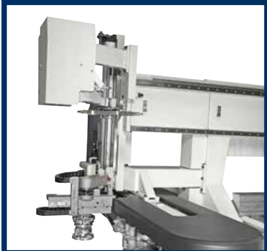
The MACH 5 device performs a tool change in just five seconds, drastically reducing downtime time.
