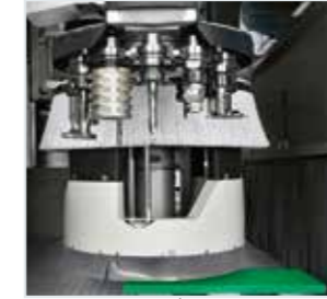
Excellent cleanliness of the machine and its surroundings thanks to the dual coaxial suction hood, which can extract chips and dust under all working conditions.
