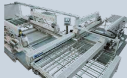
"Futura P55/26" machining centre for structural and interior glass walls, arris grinding and standard grinding
